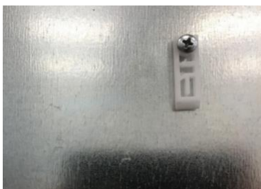
Figure 20: Top DIN Clip is shown mounted first to avoid any metal shavings from dropping in to the case.
