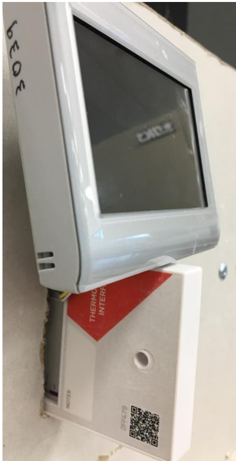
Figure-12: Replace the Thermostat face. Do not insert the Thermostat Interface into the wall until the Equipment Interface is installed and all system functions have been tested.
