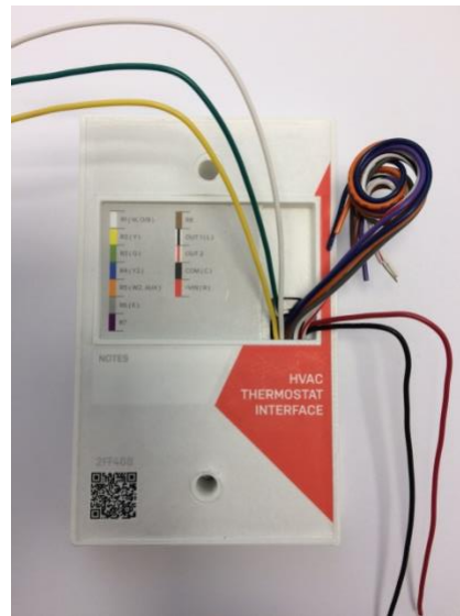
Figure-10: Following the Wire Function & Color Chart in Figure-6 (page-9), select the wires needed for the Thermostat functions required.
