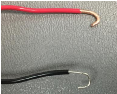
Figure-10: Following the Wire Function & Color Chart in Figure-6 (page-9), select the wires needed for the Thermostat functions required.
