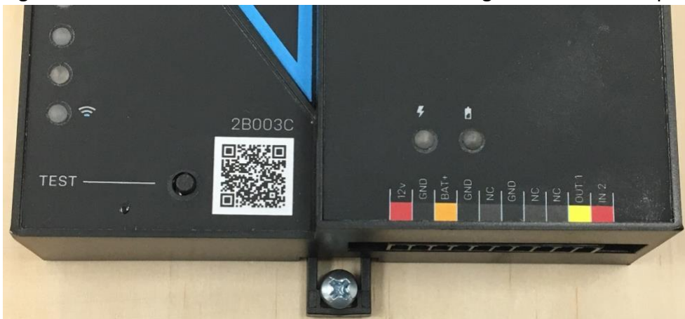
Figure 8: The bottom screw is shown mounted through the black DIN clip to the wall:
