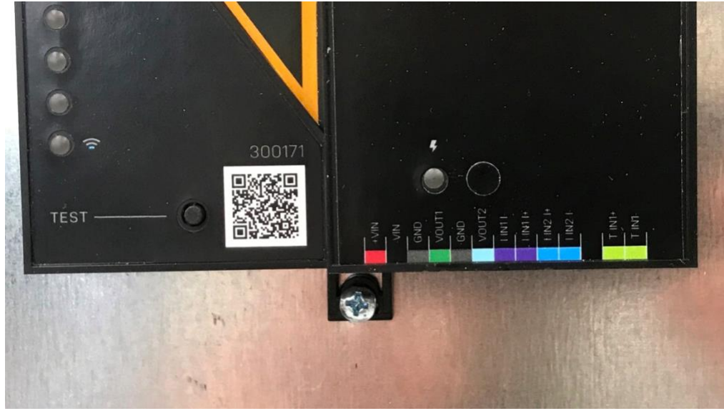
Figure 5: The bottom screw is shown mounted through the bottom DIN clip to the wall:
