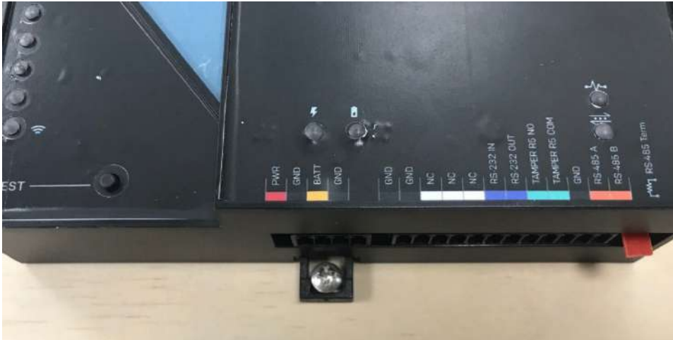
Figure 11: The bottom screw is shown mounted through the black DIN clip to the wall (Serial Pro Shown, form factor is the same):
