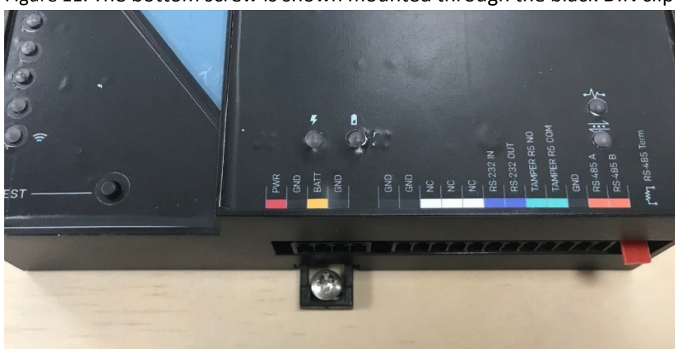
Figure 11: The bottom screw is shown mounted through the black DIN clip to the wall:
