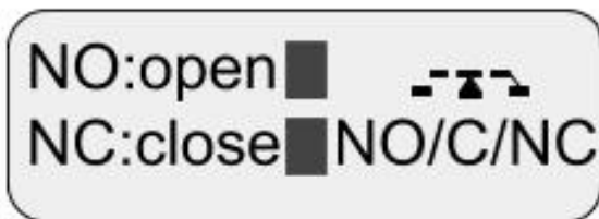
Figure 9: Relay test screen shown in which the relay NC terminal is measured as 'close' (shorted) to the relay COM terminal indicating that the relay is in the non-energized state.
