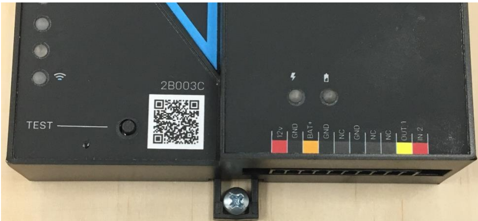
Figure 7: The bottom screw is shown mounted through the black DIN clip to the wall:
